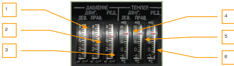
6-57: Transmission and engine oil pressure and temperature gauges
