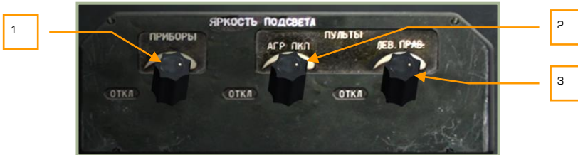
6-72: Lighting brightness control panel
