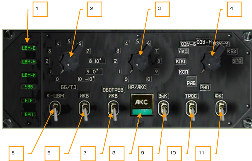
6-69: System preparation and check panel
