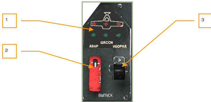
6-29: Gear control panel
