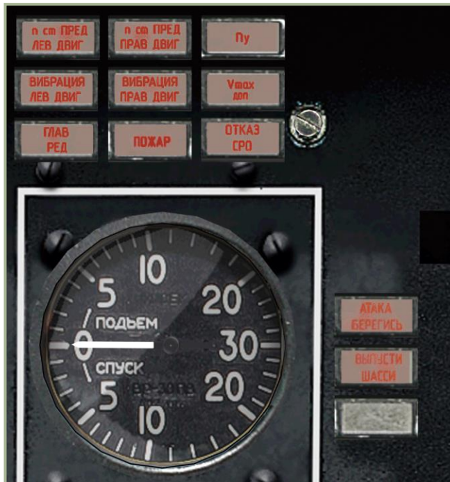
6-28: Caution light panel
