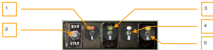
6-49: Signal flare control panel
