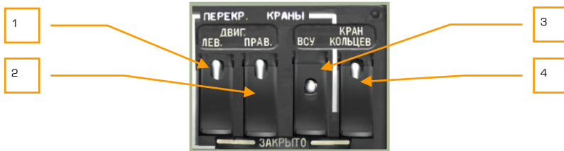
6-56: Fuel shutoff valve control
