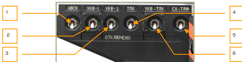
6-53: Radio and data link power control panel
