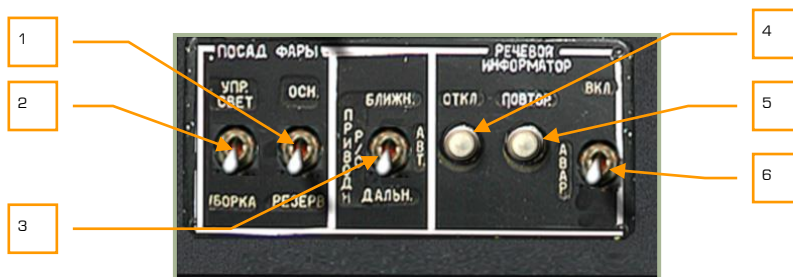
6-41: Landing lights and voice warning ("Betty") control panel.
