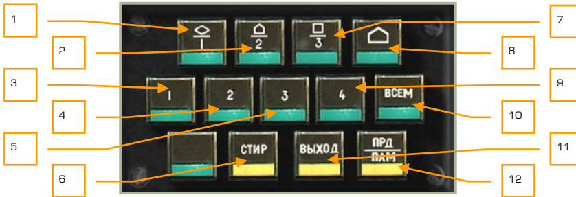
6-32: Data link control panel
