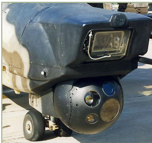
1-12: Ka-50Sh nose with "Shkval" system above and Samshit-50 optoelectronic system below
