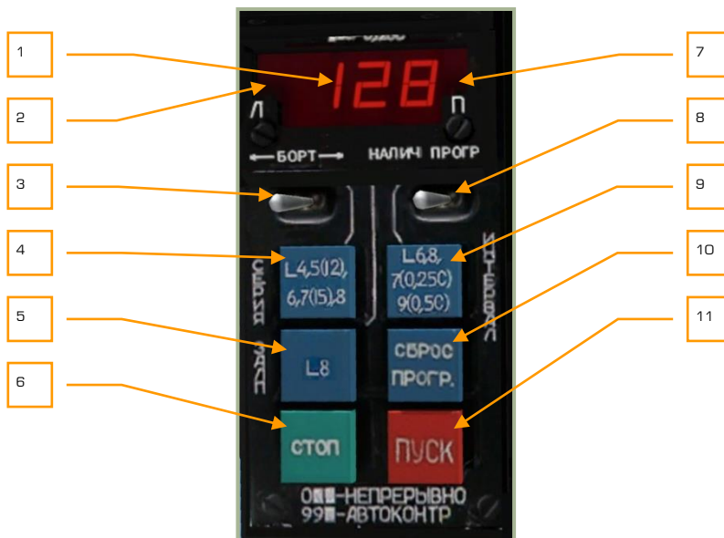
6-34: UV-26 Countermeasures control panel
