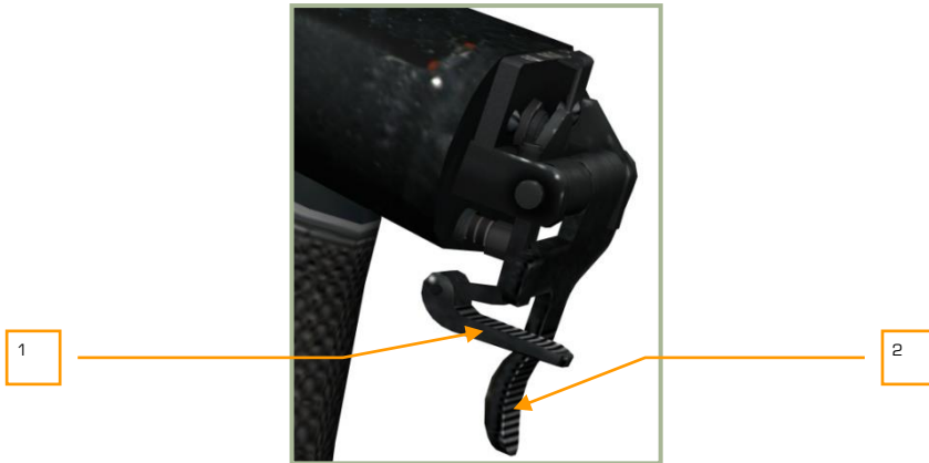
6-5: Weapon (large) and Cannon (small) triggers in default position – Release Weapon trigger operates
