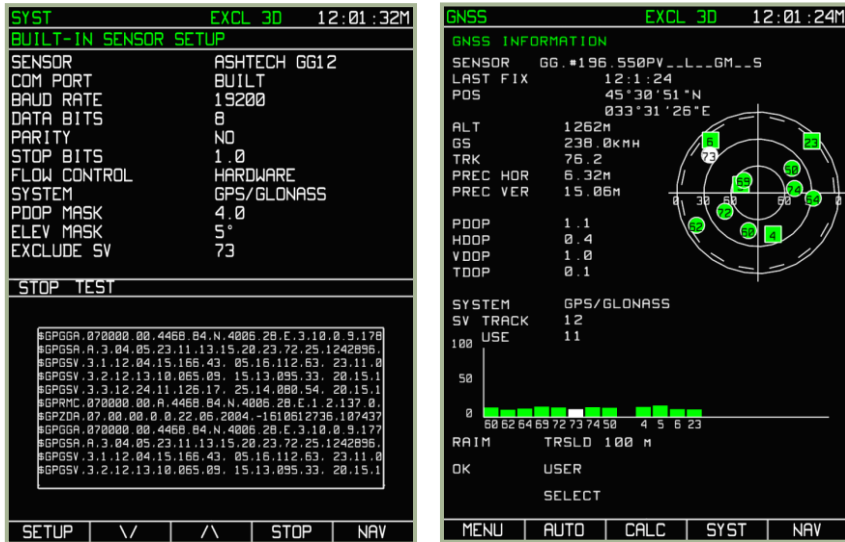
7-101: SYST page during testing of the GNSS sensor and its communication channel
