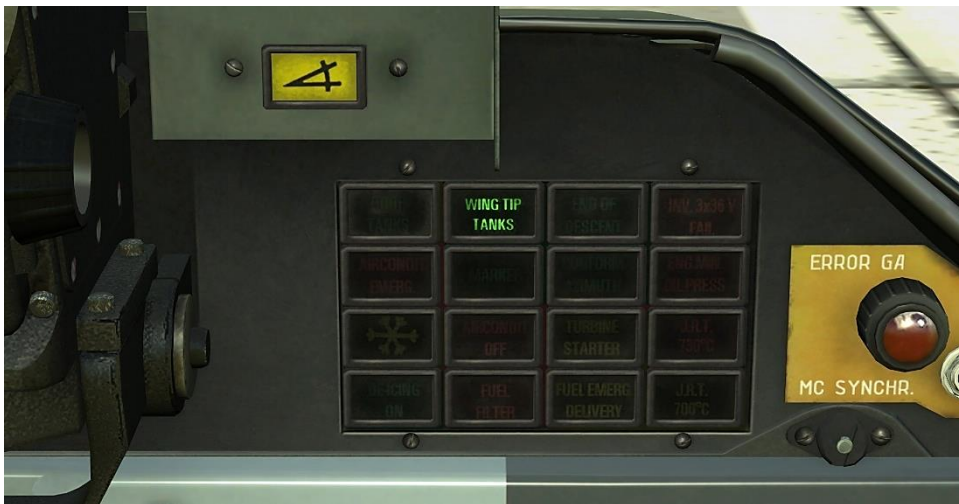
Figure 175: The WING TIP TANKS annunciator panel
