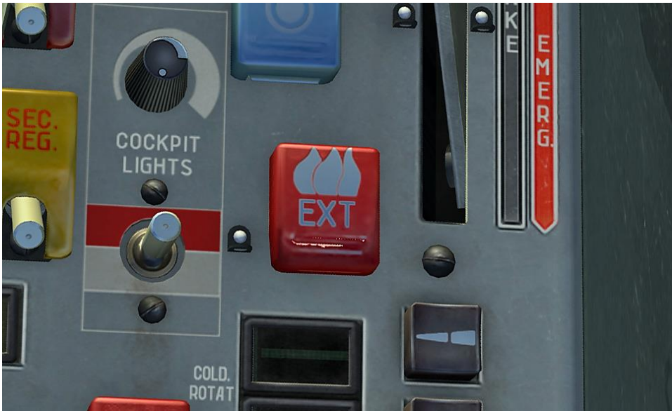
Figure 68: Fire extinguisher button
