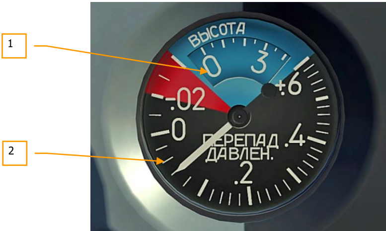
Figure 110: UVPD cockpit altitude and pressure difference gauge
