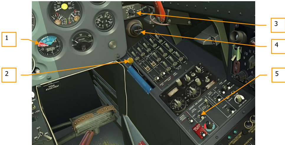
Figure 61: Air system and environmental control system controls and indication, front cockpit
