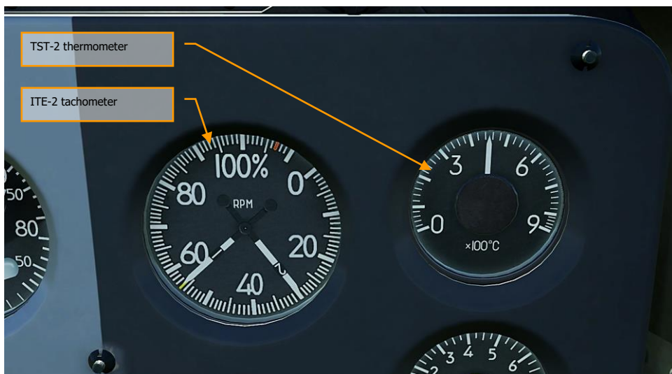
Figure 81: ITE-2 tachometer and TST-2 EGT thermometer gauges
