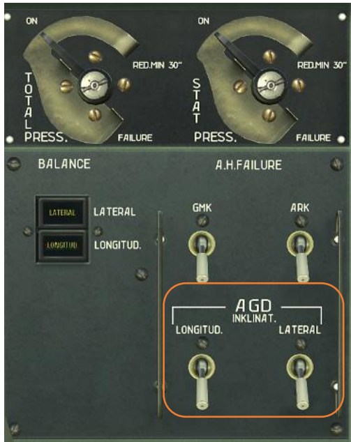
Figure 114: ADI failure simulation controls
