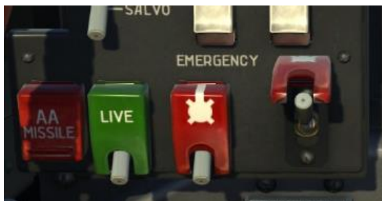
Figure 177: The EMERGENCY switch in the front cockpit
