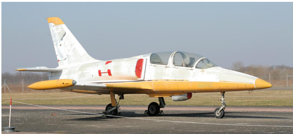
Figure 11: L-39V (Vlečná - tug) – single-seat KT-04 target tug
