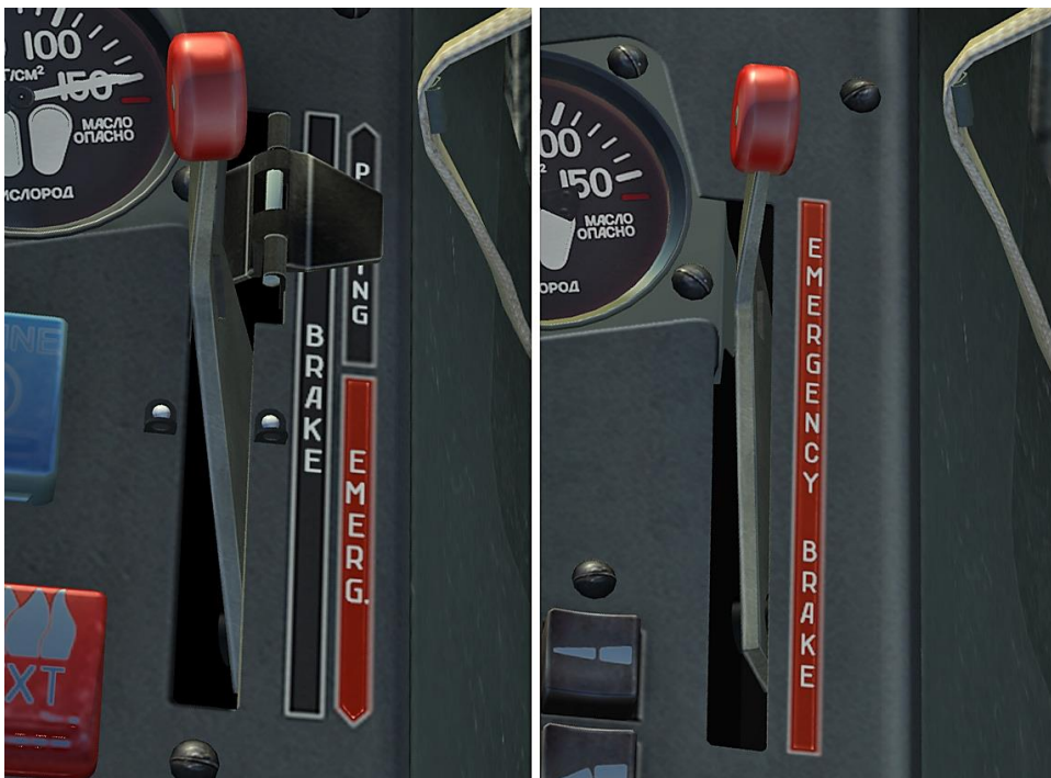
Figure 55: Emergency main landing gear braking lever, front (left) and rear (right) cockpit
