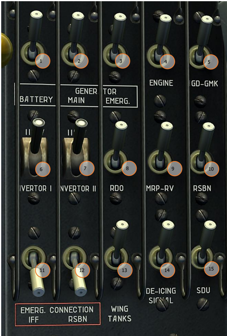
Figure 84: Main electrical CB panel, front cockpit
