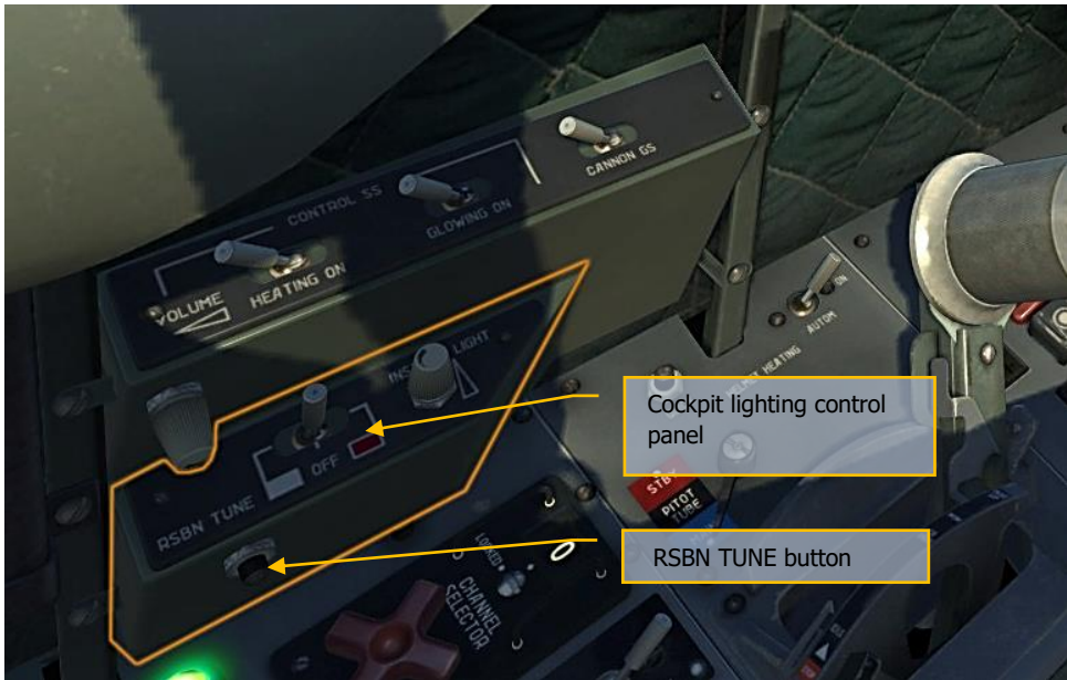
Figure 168: Cockpit lighting control panel and the RSBN TUNE button
