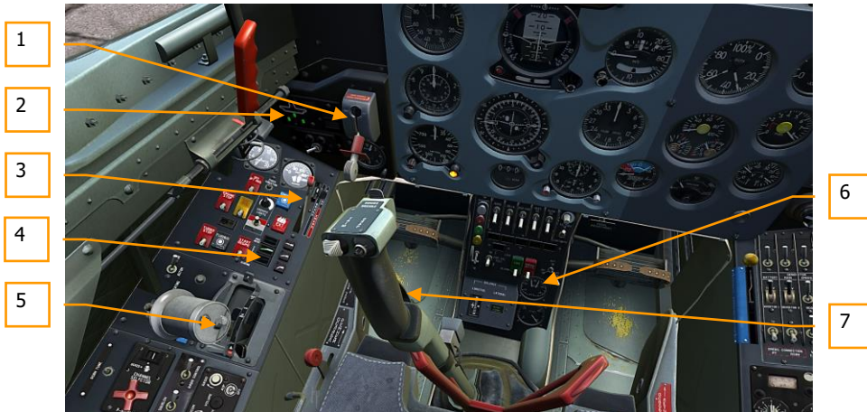
Figure 50: Utility hydraulic system controls and indication, front cockpit
