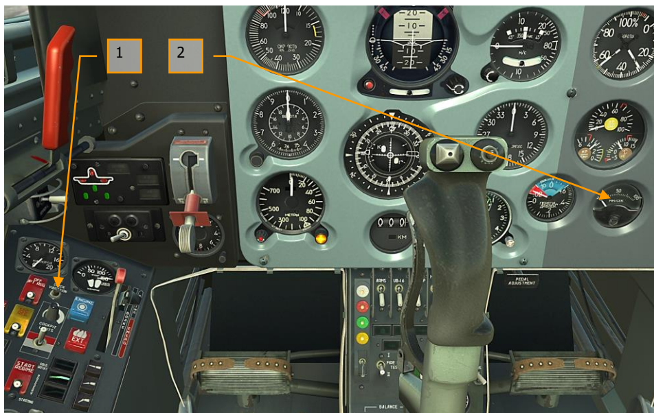
Figure 72: Vibration check controls
