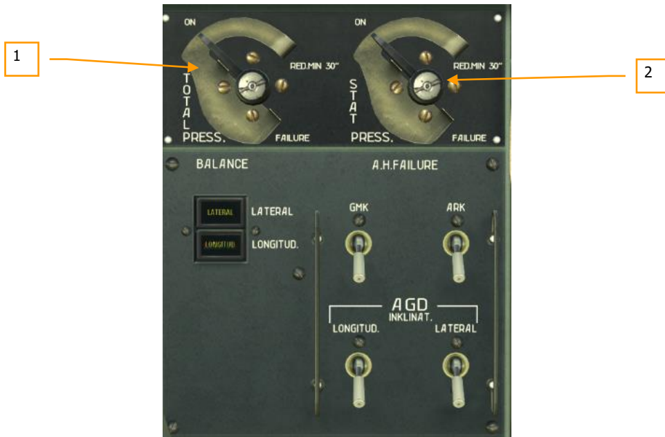
Figure 108: Front cockpit gauge fault simulation panel
