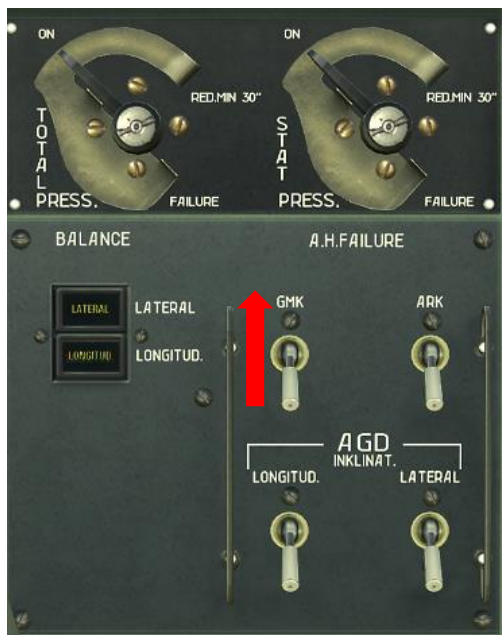
Figure 123: Control of GMK-1AE failure simulate
