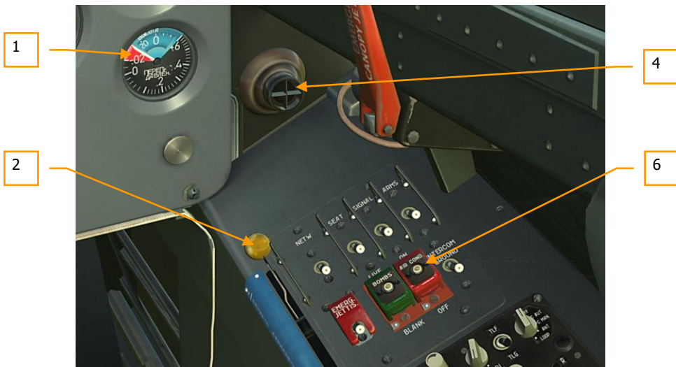
Figure 62: Air system and environmental control system controls and indication, rear cockpit
