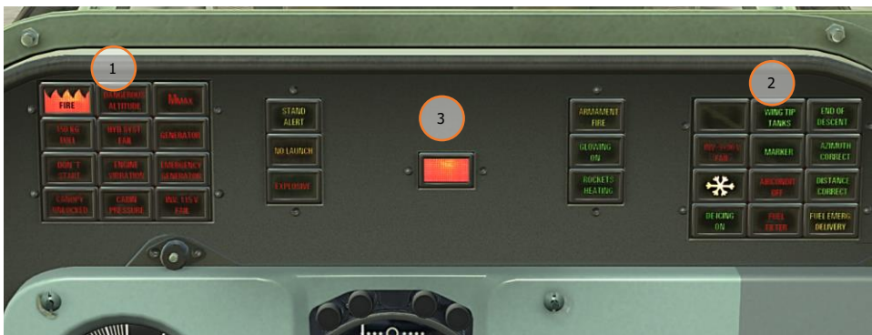
Figure 96: Warning lights and caution & advisory lights panels, rear cockpit
