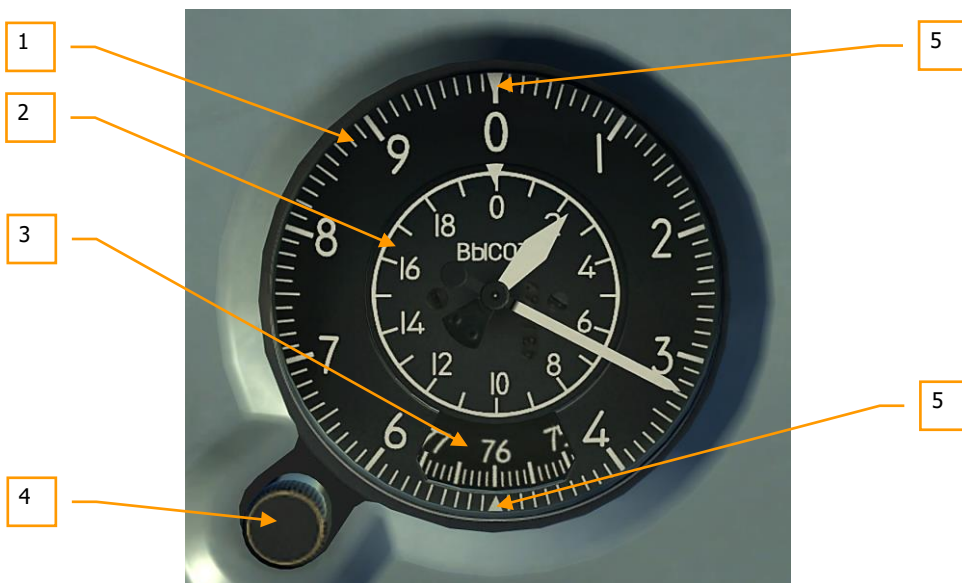
Figure 109: VD-20 barometric altimeter
