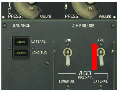
Figure 134: RKL-41 failure simulate switch
