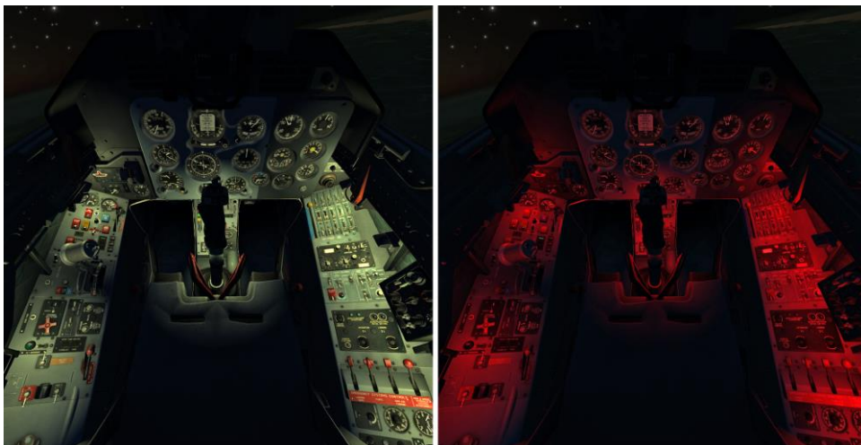
Figure 92: White and red floodlight, front cockpit
