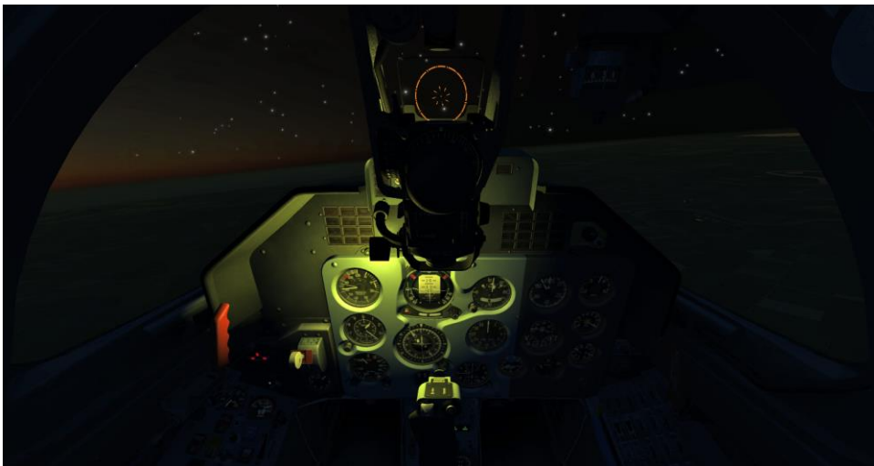
Figure 94: Cockpit with activated instrument panel emergency light
