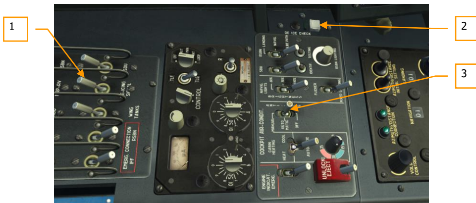
Figure 70: Anti-icing system control
