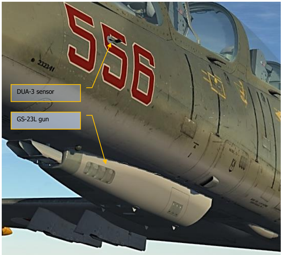
Figure 165: L-39ZA AoA sensor and gun
