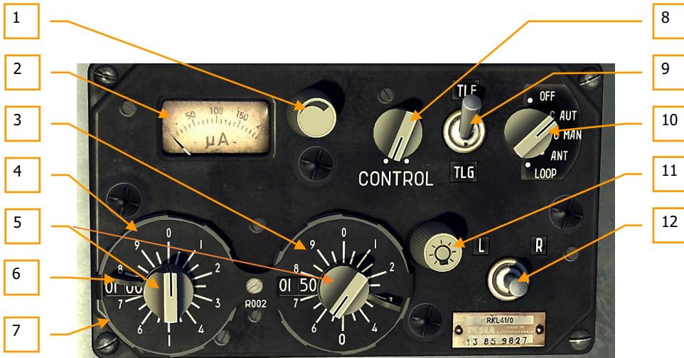
Figure 133: RKL-41 Control Panel
